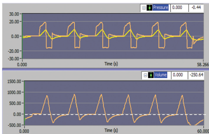
Figure 4.1: IP/EP 20 cmH 2 O with no PAP on Pause. The Expiratory Reserve Volume (ERV) is 0 mL above lung Residual Volume (RV), which predisposes patients to alveolar collapse following each cough maneuver.
